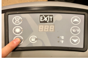
5) Connect the pump unit then press the button to inflate the spa. The air flow valve prevents your spa from over-inflating.
